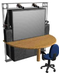
**Figure 1. The VIRTUE immersive videoconferencing station. Four cameras observing the local participant are mounted around the screen.**
